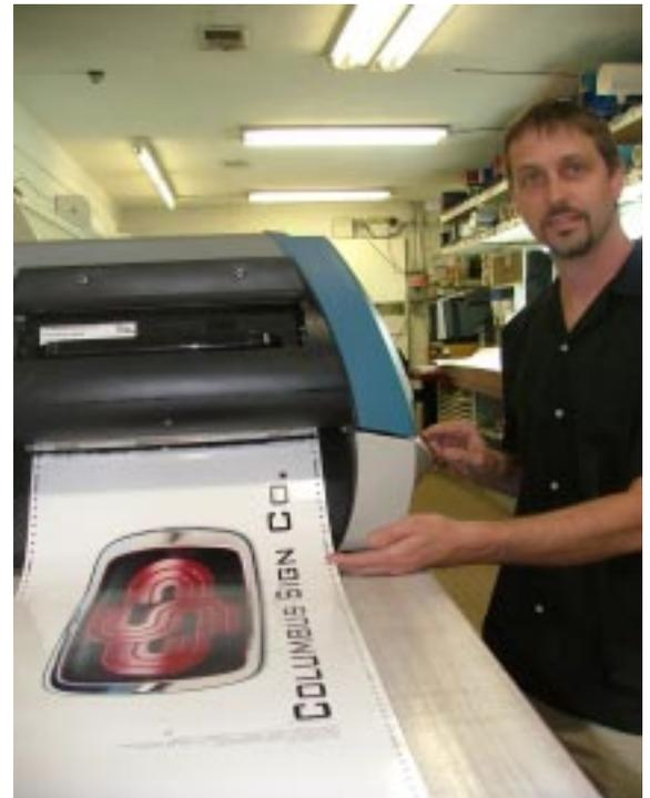
The Gerber EDGE FX is seen here printing on Gerber 3M Scotchcal 220 film, the only output film Columbus Sign chooses to use.
