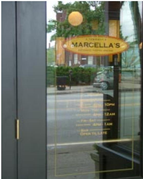
Marcella's glass door sign was EDGE printed on Gerber ImageCast clear. Before being cut out, and wet-applied to Gerber Dusted Crystal film giving it an "etched" appearance.
